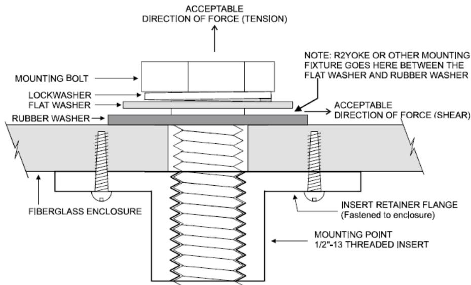
**FIGURE 3: R2 Mounting Point Loading**
