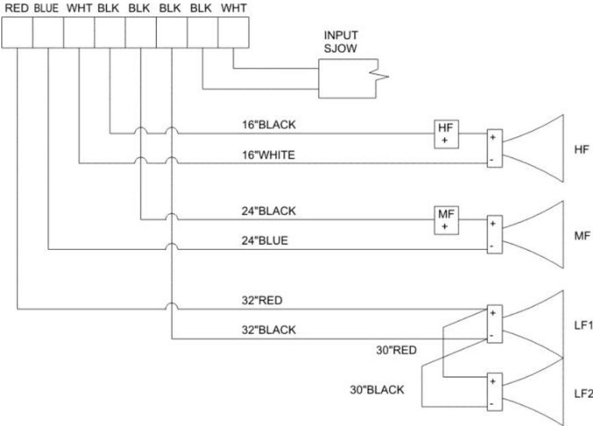
**FIGURE 6: R2 Wiring (Models R2-474Z, R2-694Z, R2-77Z and R2-94Z)**
