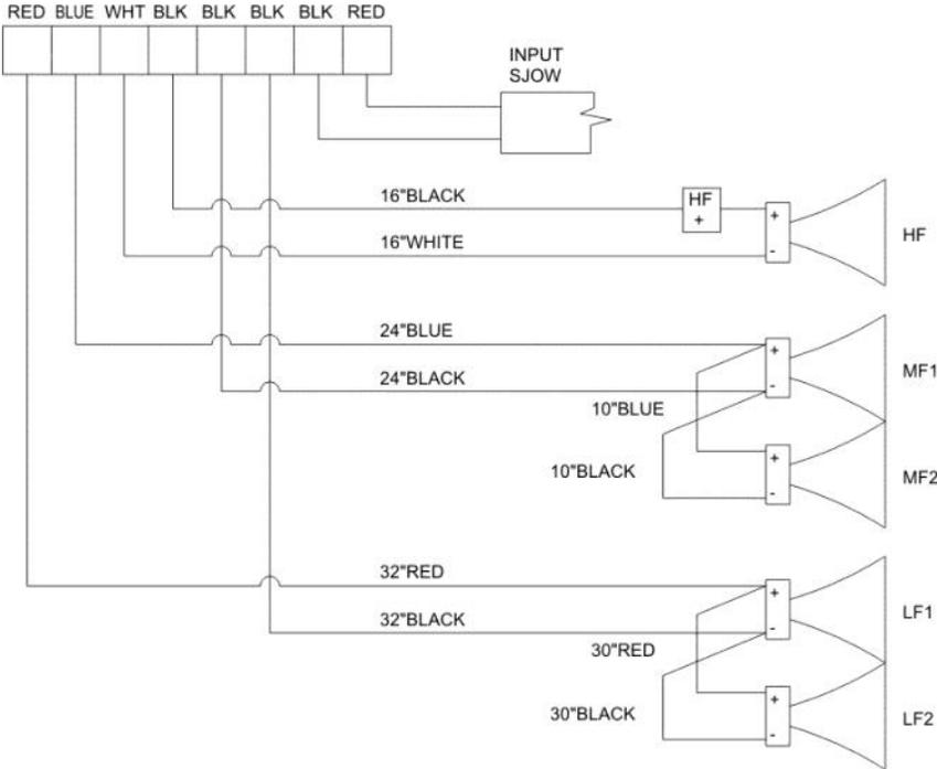
**FIGURE 7: R2-52Z Wiring**
