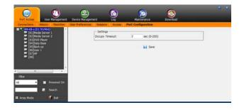
The Occupy Timeout field sets a time threshold for users on ports whose Access Mode has been set to Occupy. If there is no activity from the user occupying the port for the amount of time set here, the user is timed out and the port is released. The first user to send keyboard or mouse input after the port has been released gets to occupy the port.
