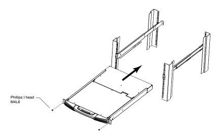
4. Slide the rear attachment sliding brackets along the slide bars until they contact the rear of the RM-KB-LCD17KVMHD, then use the screws supplied with this package to attach the bars to the rear of the RM-KB-LCD17KVMHD (tighten the screws all the way).
