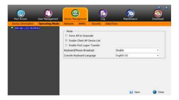
The Operating Mode page is used to set working parameters, as described below:
