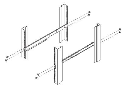
Slide the RM-KB-LCD17KVMHD onto the support flanges. Use the screws supplied with this package to loosely attach the front of the RM-KB-LCD17KVMHD to the front of the rack (only tighten the screws part way).
