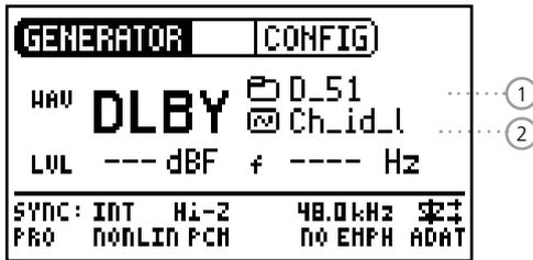
The test signals in the directories are sorted by non-linear format type.
