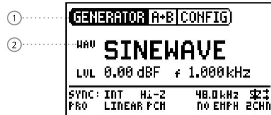
4. Select the desired test signal with the rotary wheel.
