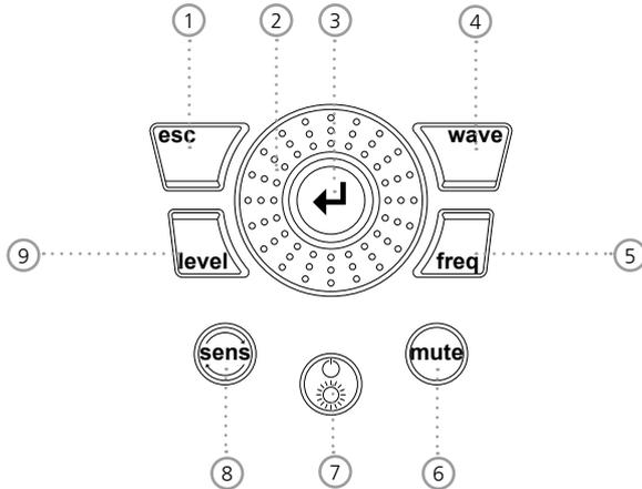
① **esc** Terminates an entry and jumps to the top menu level.
