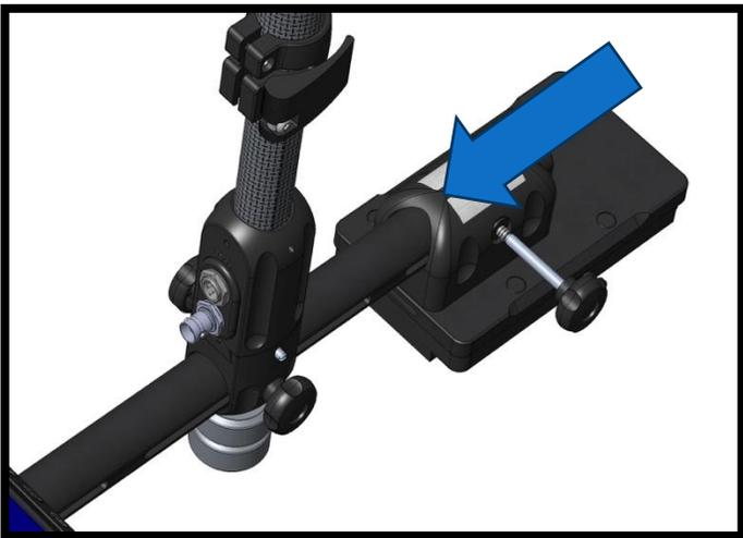
Second, remove the Battery Mount Locking Shaft, slide the Battery Mount onto the Rod and reinstall the Battery Mount Locking Shaft.
