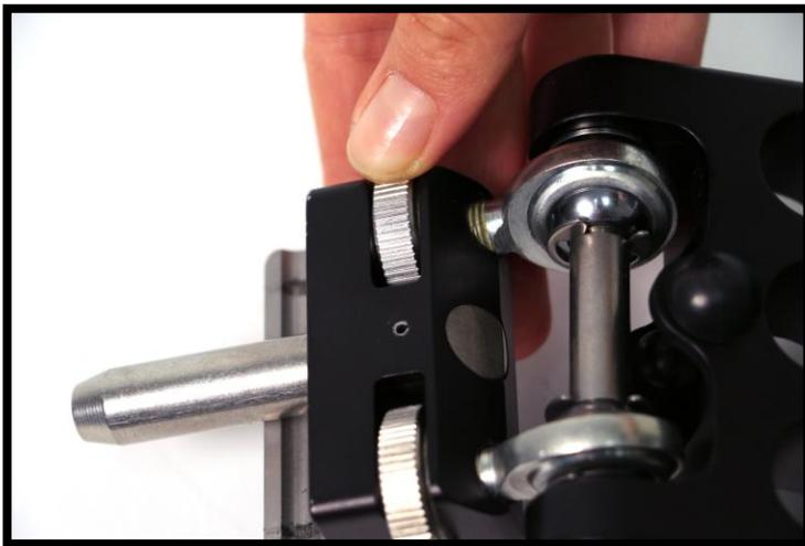
Your threads are now flipped, so reset the Side-to-Side Adjustment Wheels. Approximately 0 turns out on the bottom and 2 turns out on the top wheel.
