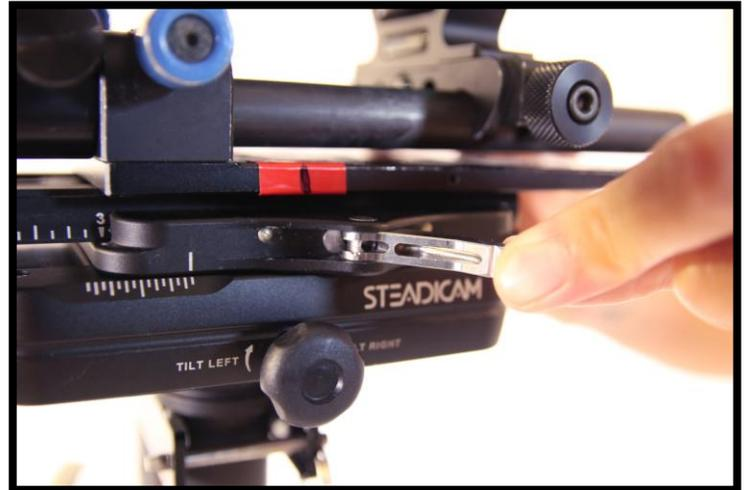
Using the Side-to-Side Knob, visually align your Side-to-Side mark with the center of the Post.
