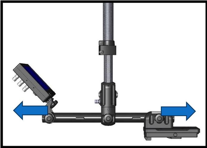
Or we can **increase** the Pan inertia by extending the masses away from the Post, making the camera more resistant to panning for architecture shots or walk and talks.
