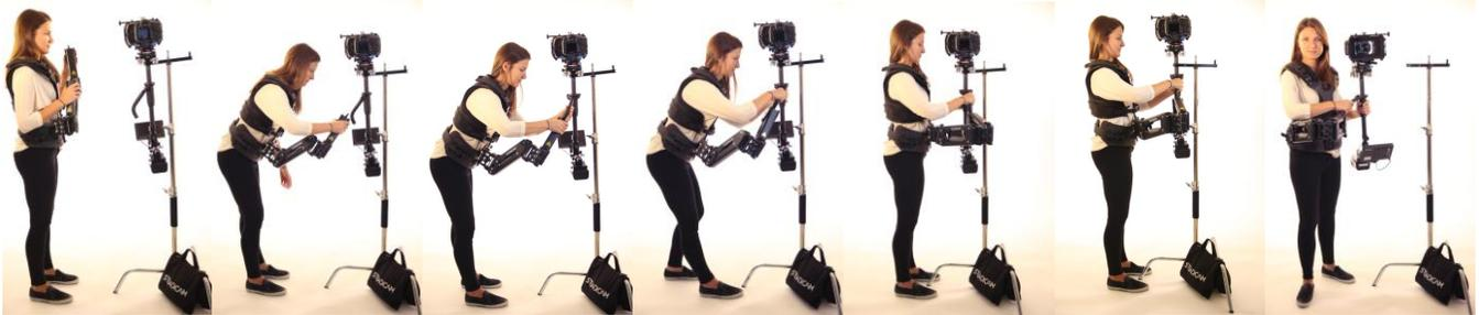
With the Docking stand raised so the Stage is roughly shoulder high, bow to the stand and place the Arm Post into the receiver of the Gimbal Handle.
