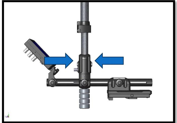
Similarly, you can **increase** the Pan inertia by extending the masses away from the center Post, including the Accessory Weights.
