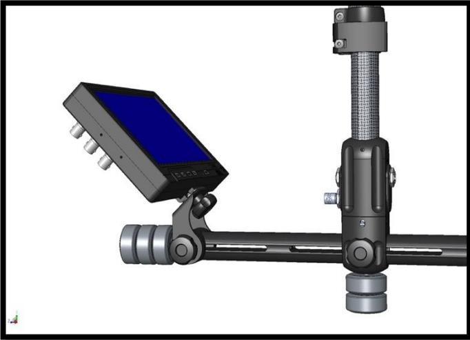
We suggest operating with the monitor at a 45° angle to the Cross Rod. This is adjustable by loosening the Monitor Mount Knob with one hand while supporting and adjusting the monitor with the other.
