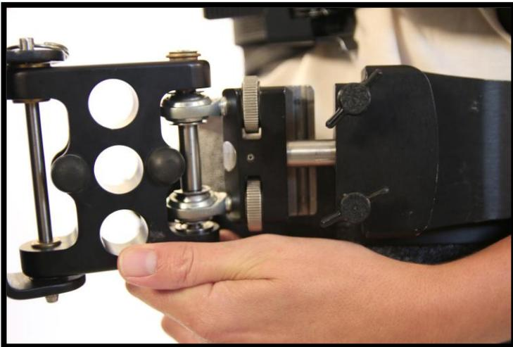
Insert the Arm Socket into the Socket Block of the Vest. Then use the Thumbscrew Bolts to secure the connection.
