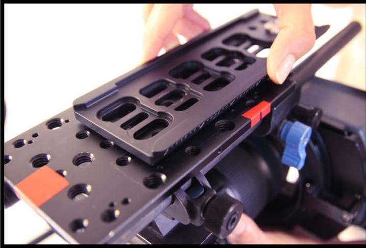
Center the camera on the Quick Release Plate using the Fore-Aft and Side-to-Side balance point marks you made.
