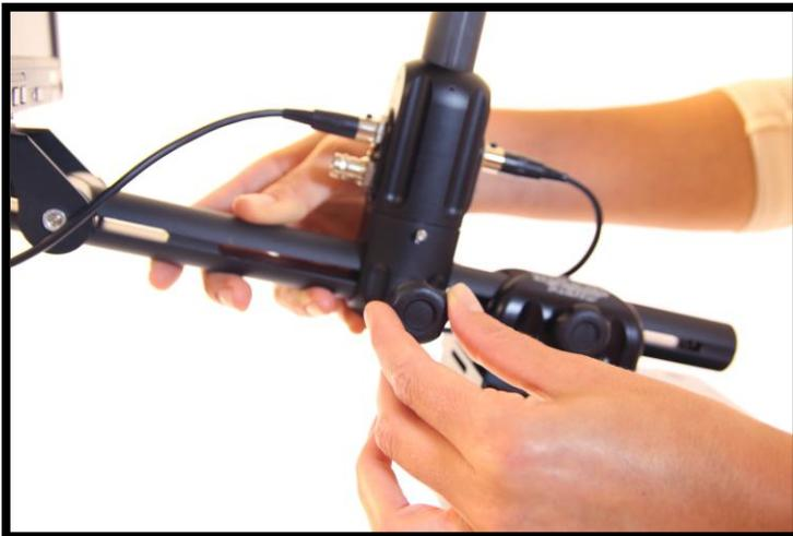
If the camera tilts significantly, loosen the Cross Rod Clamp Knob and slide the Cross Rod fore or aft until the camera remains horizontal. Then lock in the position by retightening the Knob.
