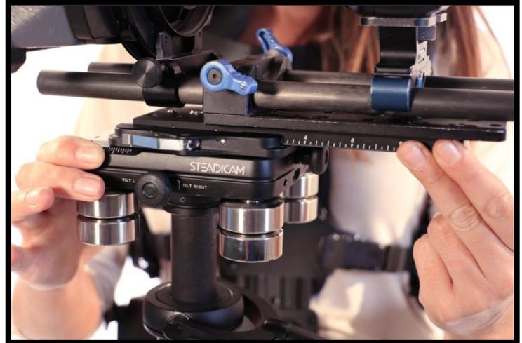
Once the AERO is in Dynamic Balance it's easy to maintain despite later changes to camera setup. As long as you only make ONE change and re-balance with that component, it'll still be in Dynamic Balance.
