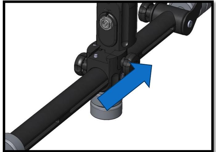
Add your choice of monitor by lining up the registration pins and attaching it to the monitor mount via the captive ¼-20 screw.
