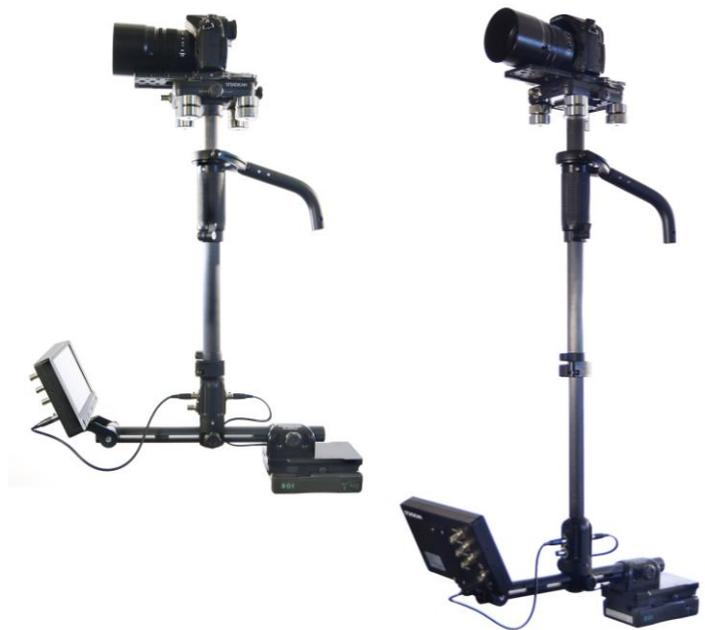
It's possible to **reduce** the Pan inertia by moving the monitor and batteries closer to the Post. This makes the camera "whippy" for action scenes or a more handheld look.
