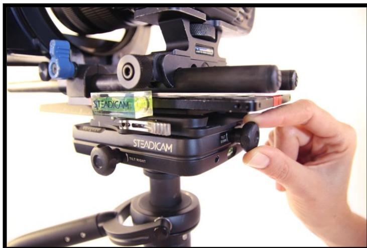
Fine tune the tilt by turning the Fore-Aft Knob one way or the other to bring the camera to horizontal.
