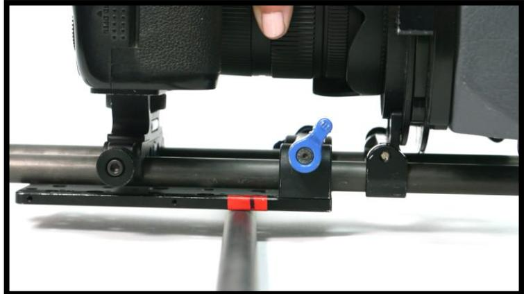
**Note:** Some camera setups, such as a DSLR with a zoom lens, may have the Fore-Aft balance point *outside* of the camera body. In this case, find the Side-to-Side balance first, and then mount the Quick Release Plate to the camera and use the base of the Plate to find the Fore-Aft balance point.
