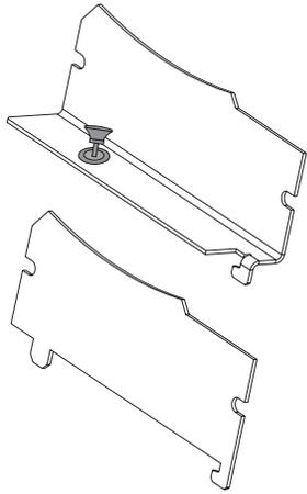
Your DA-506BID is supplied with extra mounting ears. These allow the DA-506BID to be mounted in any OpenHouse™ structured wire grid system.
