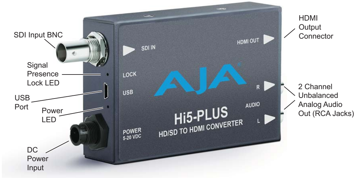
Figure 2. Hi5-Plus Converter Connections
