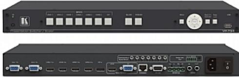
VP734 is a 7input presentation switcher/scaler with four HDMI, one DisplayPort and two userdefinable (universal) analog video inputs. It up and downscales to selectable graphics or HDTV output resolutions (up to 4K30 UHD) and provides fast fadethrblack switching between sources. VP734 supports analog and embedded audio inputs and outputs and includes rich audio functionality and a stereo loudspeaker output
